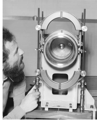
Figure 7: Scientists installing a new automatic clamp for a beam line in the North Area in 1978 (Copyright: CERN) [12].
